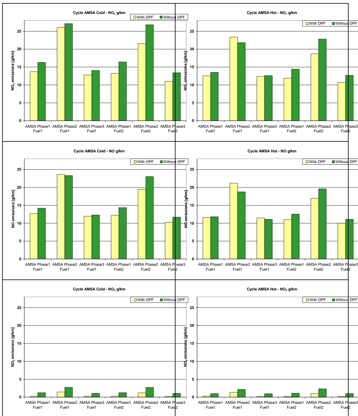
Fig. 12 – NO x , NO and NO 2 emissions over the AMSA driving cycle (cold-hot) for both tested fuels.
