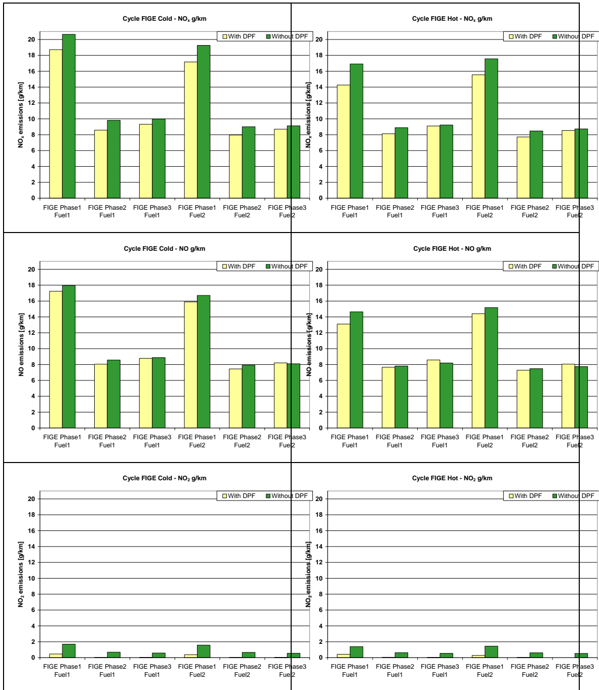
Fig. 9 – \text{NO}_x , NO and \text{NO}_2 emissions over the FIGE driving cycle (cold-hot) for both tested fuels.
